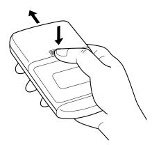
2 Replacing the battery Put the batteries in the case observing the polarities as illustrated.
